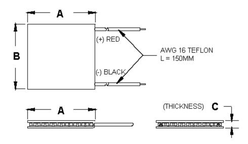
Ceramic Material: Alumina (Al<sub>2</sub>O<sub>3</sub>) Solder Construction: 138°C, Bismuth Tin (BiSn)
